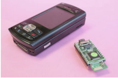
Figure 3: A mobile phone and wirelessly integrated Bluetooth module for supporting analogue and digital I/O
